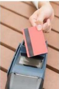
The underlying technology, commonly referred to as near field communication (NFC), enables the contactless use of a card or mobile phone. During a contactless transaction, information is exchanged and transmitted via a radio signal between the card or mobile phone and the payment terminal.
