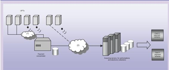
UPTs installed on the merchant's premises, such as, for example, automated fuel pumps at a fuelling station, are generally connected to an aggregating device known as the payment concentrator, which receives data about payment transactions conducted on the terminals and provides the link to the acquiring server(s). The server then sends authorisation requests and electronically collected data to the relevant card payment scheme(s).
